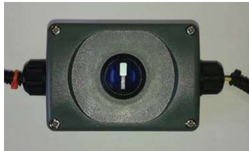
Figure 33 — Hatch Selector Switch
