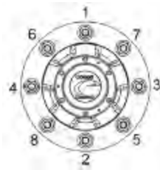
Figure 55 — Order for Tightening the Nuts
