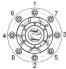
Figure 62 — Order for Tightening the Nuts
