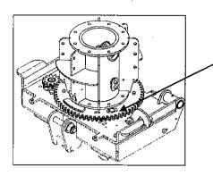
1- The turntable locking key must be in line with the turntable slot
