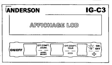
To start the counter press the **ON/OFF**TSK (Touch sensitive key), which will bring-up he first display. **Anderson**. After 5 seconds the following information will appear in the window:
