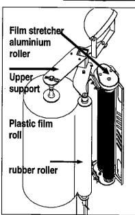
To remove an empty film roll lift up the spring loaded top plastic film guide and slip out the bottom end of the empty roll. To install a new plastic film roll insert the top center of the film roll in the spring loaded film guide and slip back-in the bottom end of the plastic film roll and feed the plastic film through the rubber and aluminum stretch rollers as shown in figure.
