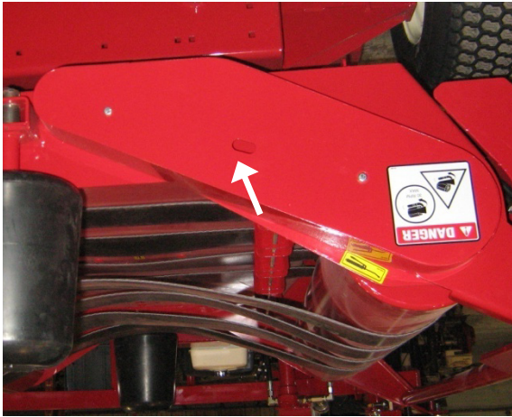
Figure 6.2 Lubricating the plastic film stretcher
