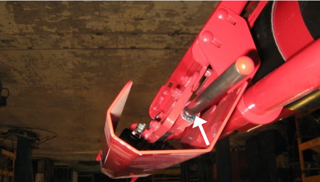
Figure 6.4 Lubricating the plastic film cutter 1
