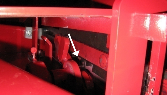
Figure 6.4 Lubricating the plastic film cutter 1
