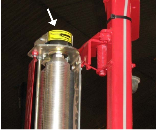
Figure 6.2 Lubricating the plastic film stretcher
