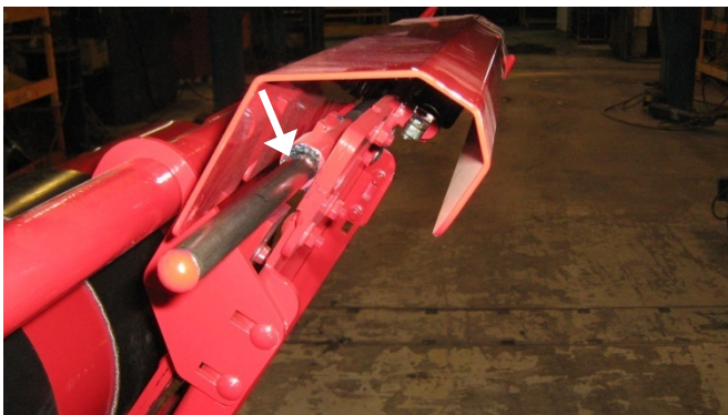
Figure 6.4 Lubricating the plastic film cutter 1
