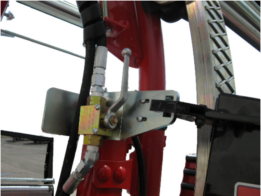
Figure 13 – Valve du frein
