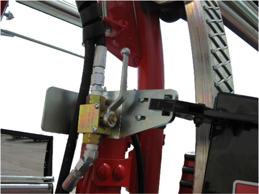
Figure 13 – Valve du frein
