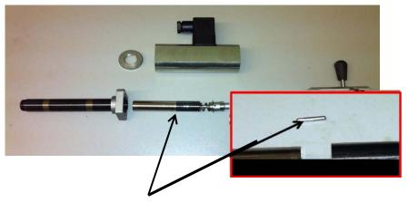
5- Remove the small pin and then remove piece by piece.
