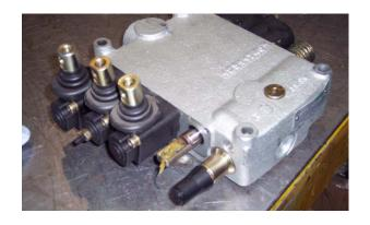
3- Remove the spool toward the back, VERY IMPORTANT: remove the 2 o-rings on the front and on the back. Pay attention on the assemble order.
