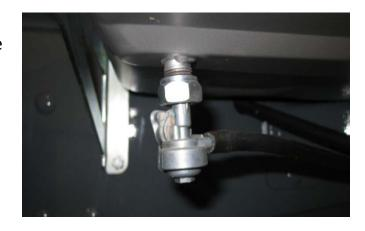
3- Install 3 way gas valve as close as possible of the Honda motor. You may have to drill holes to fix the bracket.
