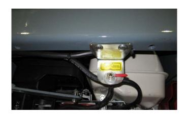
4- Install the hoses for the tank. When installing the long hose from the large tank bring it back around the back of the oil tank of the wrapper so that it is away from moving parts under the wrapper.
