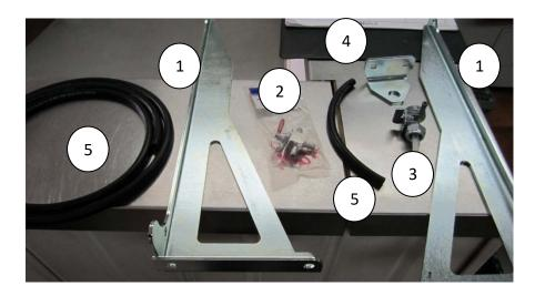
1- First step is to install the gas tank brackets on the frame. You may have to drill holes. On newer machines, holes will be there already. The tank must be installed on the back left side of the machine (see photo).
