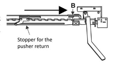
Put the last bale to be wrapped on the wrapper and when cycle is completed make sure that the bale is not on the pushing head of the X-Tractor. The system will be ready to use and you'll avoid any damage to the X-Tractor cylinder.
