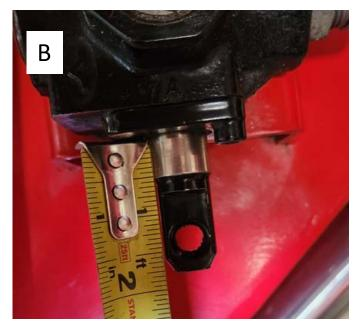
If the spool of one of its valves is stuck in the in position (image A), but the units are raised, you can pull on the spool in order to free it. Afterwards, make sure it moves easily (exiting and entering). If the spool moves with difficulty and tends to get stuck, change the valve.
