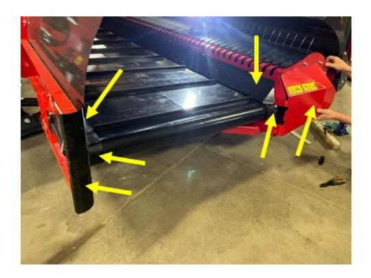
29- Adjust the plates to ensure there is at least  $\frac{1}{4}$ " of space everywhere between the plates and the belt.
