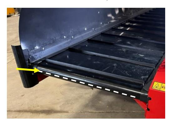
5- Push the traction roller as far inwards as possible. Remove the pin from the belt tensioner system to complete this step.
