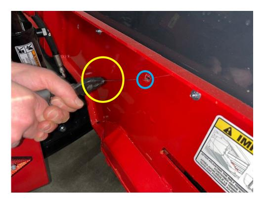
23- Stop pulling when the sheathed hook is at the edge of the belt.
