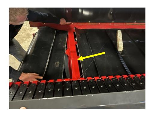
12- Make sure the new lace is at least twice the length required to cover the width of the belt.
