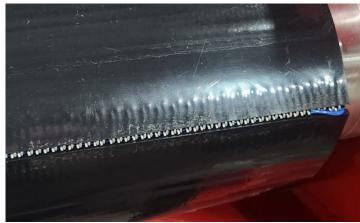
26- Align the guide under the belt in the center of each traction roller.
