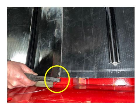
19- Lubricate the alligator seal in a small amount. Do not lubricate the section of the lace which is not yet entered, you pliers may slip.
