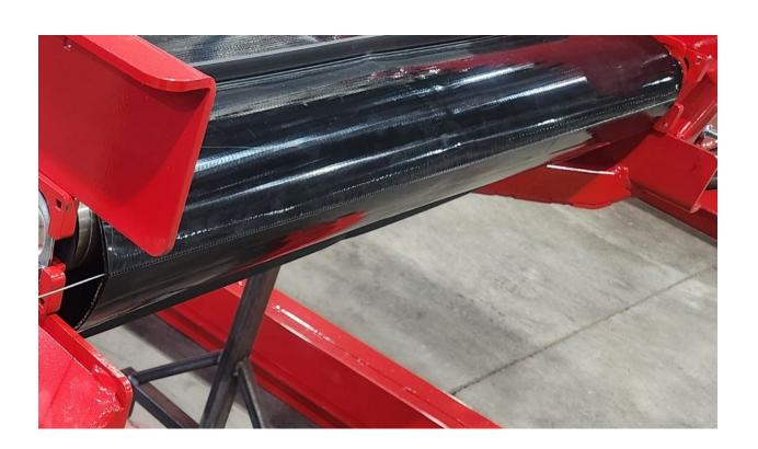
19- Enter the lace on the unsheathed side at the same time as the other person pulls on the wire (lace tool) to remove it. For efficient work, make sure the lace enters at the same speed as the wire (lace tool) exits.
