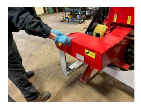
14- Make a clean cut in the sheath to avoid any fraying.
