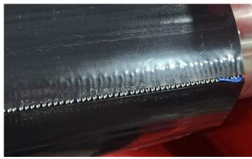
24- Align the guide under the belt in the center of each traction roller.
