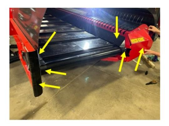
27- Adjust the plates so that there is a minimum of  $\frac{1}{4}$  inch of space everywhere between the plates and the belt.
