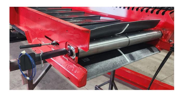
12- Make sure the new lace is at least twice the length required to cover the width of the belt.
