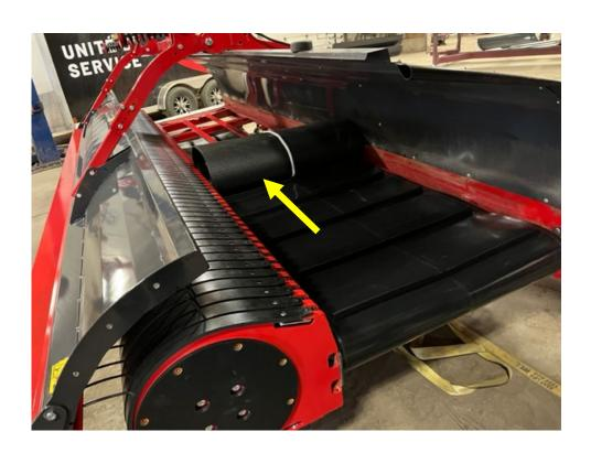
11- Place the belt joint over the pulley on the belt adjustment side (outer side of the unit).
