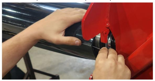
20- If necessary, use pliers to push on the lace. Make sure it comes out the other side, being careful not to bend the lace.
