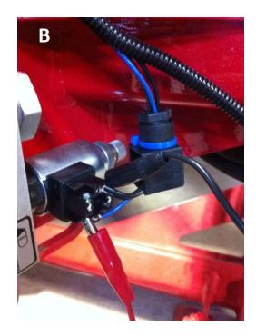
When your voltmeter is connected you can run the machine in Automatic mode and watch the voltage. If the voltage going to the valve is ok, you may need to check the spool or replace the valve. Be sure that the screw at the end of the spool is unscrewed totally. If there is no Voltage going to the valve you need to check the wire harness going to it and the computer.
