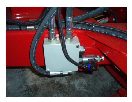
This valve controls the flow of the oil throughout the hydraulic system. When in manual mode (using the levers of the machine) this valve is fully open. When in automatic wrapping mode, the computer sends a specific current to the solenoid of the valve to push the spool into the valve and limit the hydraulic flow for different stages of the wrapping cycle. These stages are noted below with their approximate flow (voltage sent to valve).
