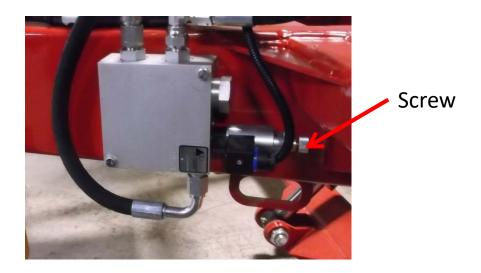
If you have received Hydraulic Error on the remote control and you have already verified the encoder, the hydraulic fluid level and the battery of the wrapper; also the machine works well manually you may have a problem with this valve. The next section shows you how to check the voltage going to the solenoid of the proportional valve. This will allow you to find the problem in this system. Whether it be with the computer, the electrical connection going to the valve or the valve itself.
