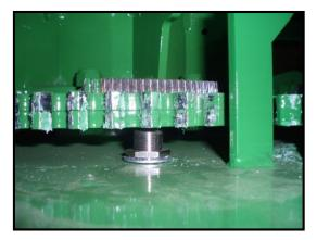
This sensor reads a hole in the main gear of the turntable. This tells the computer when the table is at point zero position. Be sure that the hole in the gear is free of grease and metal filings. In order to get a reading from this sensor you will have to turn the table of the wrapper. When it gets to the hole in the table it will shut out the indication light for a second in the computer box and at the end of the sensor.
