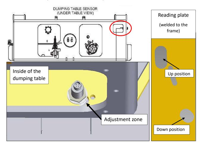
**Note:** Prior to adjust the unloading sensor, make sure the table is adjusted properly sideways. See REF# A-IND-018 Unloading Table Adjustment.
