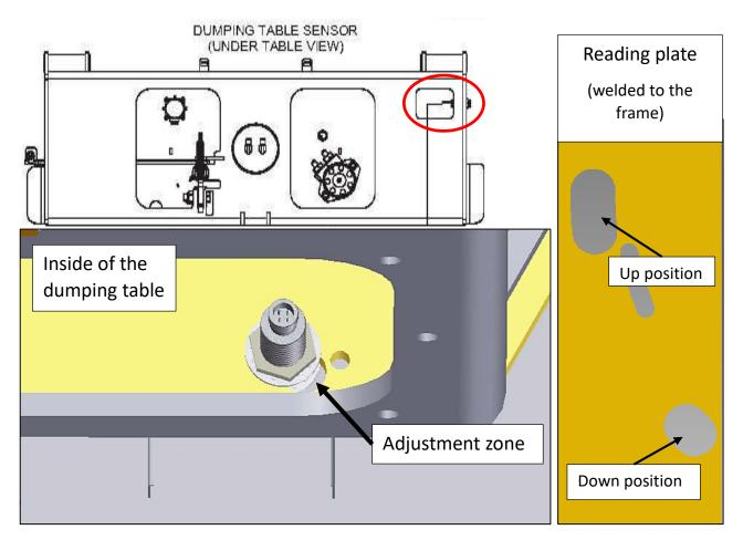
**Note:** Prior to adjust the unloading sensor, make sure the table is adjusted properly sideways. See <u>REF# A-IND-018 Unloading Table Adjustment</u>.
