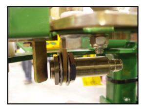
The sensor will read the metal tag as the roller on the stretcher turns.
