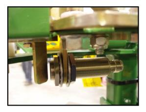
The sensor will read the metal tag as the roller on the stretcher turns.
