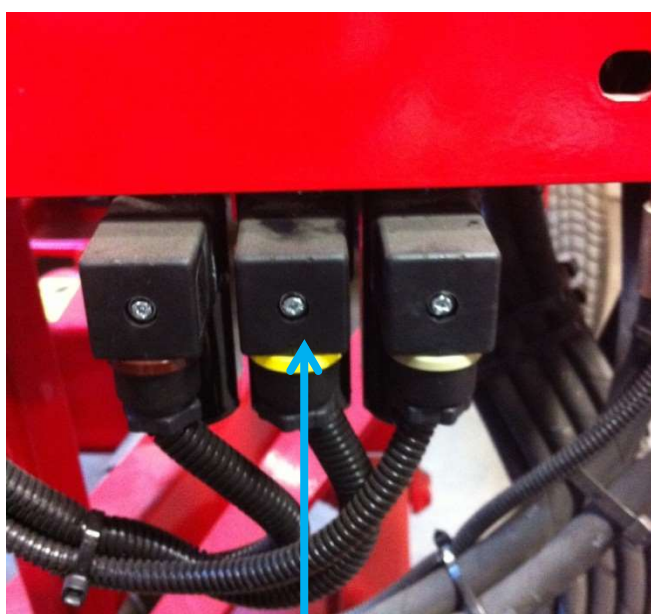
Black casing of the solenoid connector
