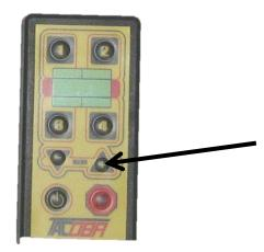
To switch from MENUS mode to programming adjustment mode (or vice-versa), simultaneously press the buttons [+] and [-], then release.
