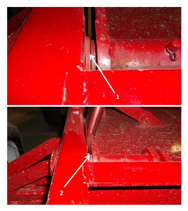
We use shim (1) on both side of the table to align the unloading table, with a pry bar (2). You are not supposed to be able to move the table more than 1/16".
