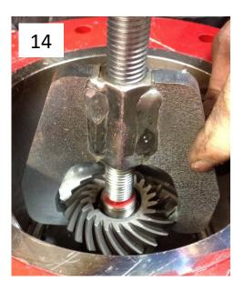
13- Remove the metal washer. Remove the bearing with the puller (#223244, photo 15) designed by Anderson Group. You have to install it and screw the adjustment (photo 16). The parts will be released together.
