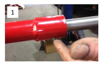
5- Remove the shear bolt (photo 2). You can now take off that piece of the shaft.
