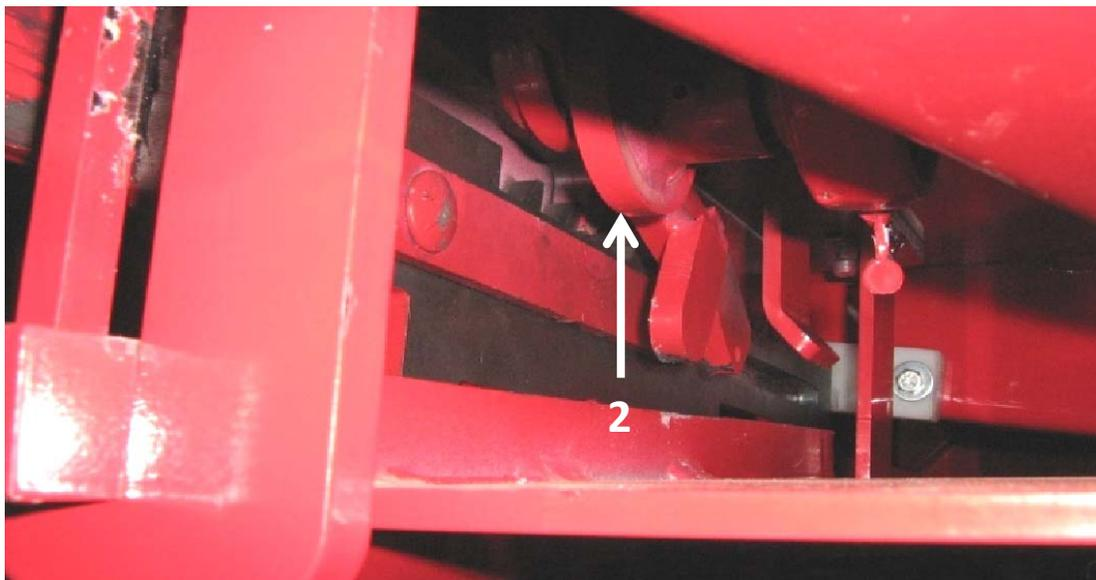
The cut & hold must be lubricated daily (approximately 100 balls) where indicated in the pictures (1 – 2). Use an antifriction lubricant to lubricate the cut & hold system. Do not use grease on the stainless steel rod because it causes an accumulation of dust that will affect the movement.
