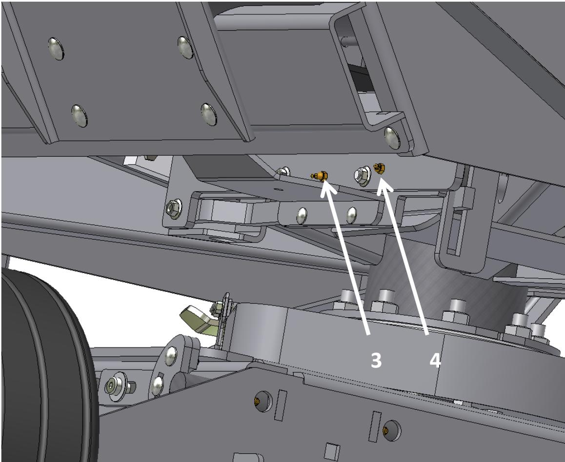
The cut & hold must be lubricated daily (100 bales) with a grease gun below the table (3 – 4).
