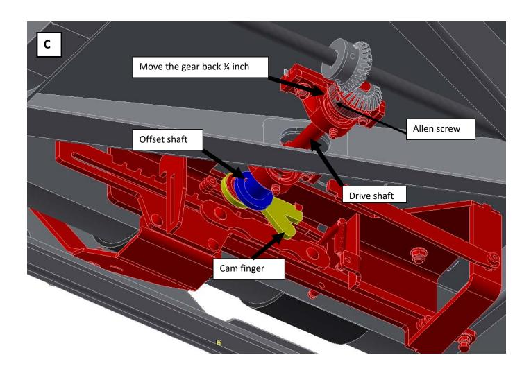
4. If the offset shaft is not in the needed position, unscrew the Allen screws (fig C) and move the miter gear back about ¼ inch on the drive shaft (fig C).
