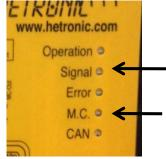
\*If the remote turns on and you don't have access to the menu, the remote and the receiver are not communicating. Consult the procedure A-IND-041 in order to clean up the remote key as well as reset this one in needed.
