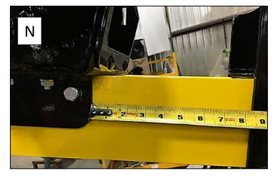
15- Install the pulley support with the provided bolts (1/2 X 4") to a distance of 8 ½" from the winch (N) with a 3/4 wrench and socket.
