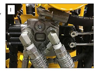
10- With a 15/16 wrench, install the provided hose #13 that goes from the main valve (G) to the option valve (J). Install the 90° elbow side hose to the top fitting of the option valve.
