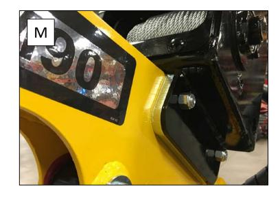
14- Install the winch on the boom facing the holes. Screw on the provided bolts (1/2 X 6") with a ¾ socket and wrench (N).
