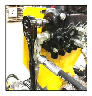
5- With a 6 mm (or 7/32) Allen socket, remove the plug (D) to the left of the previous removed fittings (step 3).
