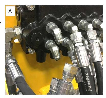
3- With a 11/16 wrench, remove the fittings (B) of the right outrigger (temporarily).
