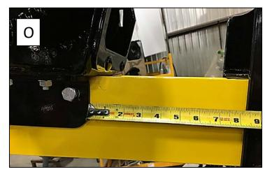
15- Install the pulley support (P) to a distance of 8 ½" from the winch (O) with a ¾ wrench. Be careful that the pulley does not hit the cylinder.
