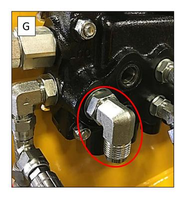
8- With a 9/16 and 11/16 wrench, reinstall the fittings of the outrigger by starting with the below one (H).
