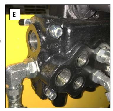
6- With a 1 1/16 wrench, screw the power beyond and the fitting at the end, if not assembly (F) in the main valve.
