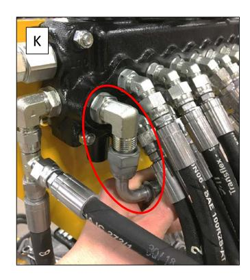
11- With a ¾ wrench, Install the other end of the #29 hose to the bottom position of the option valve (L).
