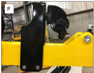
16- Screw completely the nuts(Q) under the winch with a9/16 socket or wrench.
