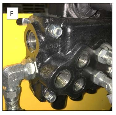
6- With a 1 1/16 wrench , screw the power beyond and the fitting at the end, if not assembly (G) in the main valve.
