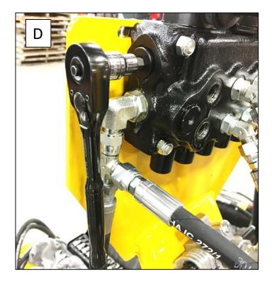
5- With a 6 mm (or 7/32) Allen socket, remove the plug (E) to the left of the previous removed fittings (step 3).
