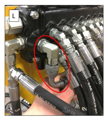
11- With a <sup>3</sup>/<sub>4</sub> wrench, Install the other end of the #29 hose to the bottom position of the option valve (M).
