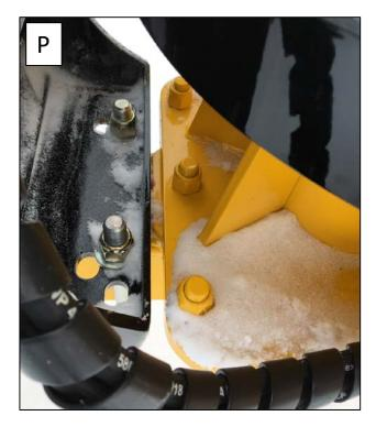
15- Install the elbow side provided hoses, to the hydraulic motor of the winch. The #22 hose goes to the top fitting and the #23 hose goes to the bottom fitting. Well attach with Ty-Rap. Install the provided hose protector (spiral guard) as showed (Q) and pass the hoses through the hole under the mast until the option valve.
