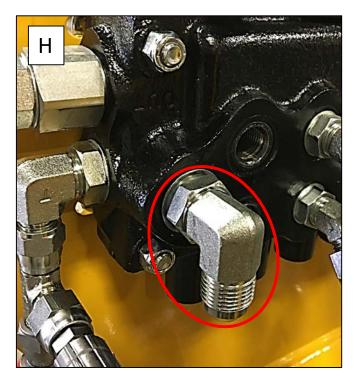
8- With a 9/16 and 11/16 wrench, reinstall the fittings of the outrigger by starting with the below one.
