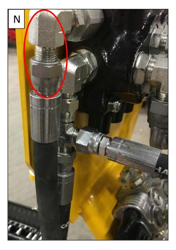
13- With a ¾ wrench, install the other end of the #28 hose to the top fitting of the option valve (O).
