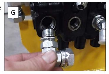
9- Reinstall the fitting of the right outrigger (H) removed earlier at step 5.
