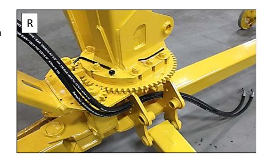
19- Connect the hoses in the motor of the winch (S) and install the U bolt to the frame. It is important to try if the valve works on the good way. Alternate the hoses if needed.
