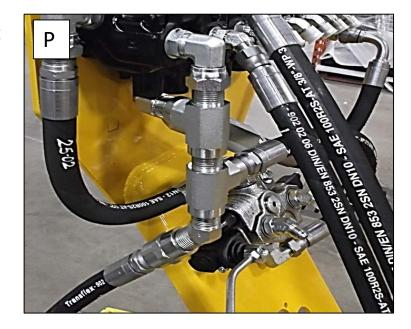
17- Install the 2 hoses #22-21 that go from the option valve to the winch (Q).
