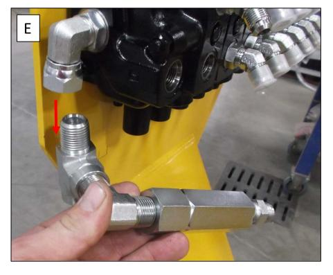
7- Install the provided plug (450062) deep inside the hole of the main valve (F).
