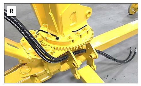
19- Attach the winch base temporarily to the frame with the U bolts (by fingers). Screw definitively the provided bolts that holds the winch to the base.
