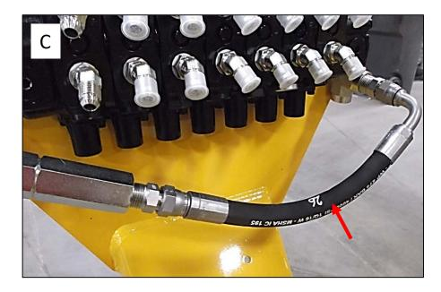
5- Remove the plug (D) and put in the garbage. Unscrew temporarily the lower fitting of the right outrigger.
