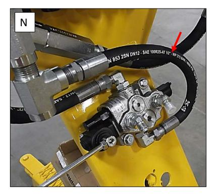
16- Install the remaining fittings (O) the way it faces the front of the log loader in order to well install the return hose to the tractor (P).
