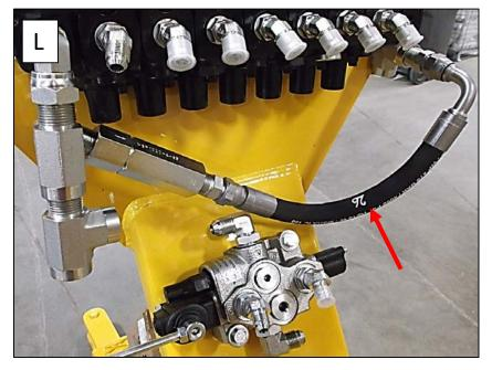
14- Install the #25-02 hose from the main valve to the top fitting of the option valve (M).
