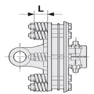
If the machine will not be used for several weeks, particularly if it will be stored in a humid environment, unscrew the springs and remove the disks to prevent them being stuck for future use.
